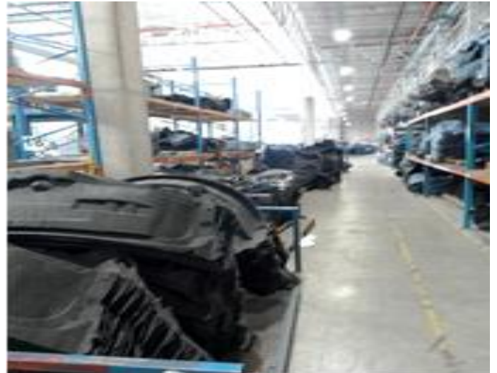
Feltex Building: Bad Housekeeping; Empty Boxes Adding To The Fire Load
