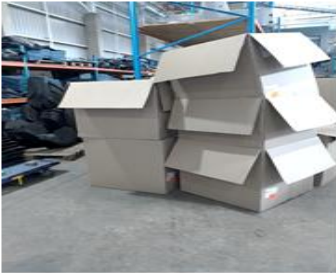
Feltex Building: Bad Housekeeping; Empty Boxes Adding To The Fire Load
